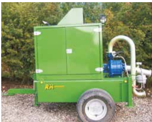
With Acoustic Canopy shown with suction extension, gooseneck delivery and control panel in enclosure
